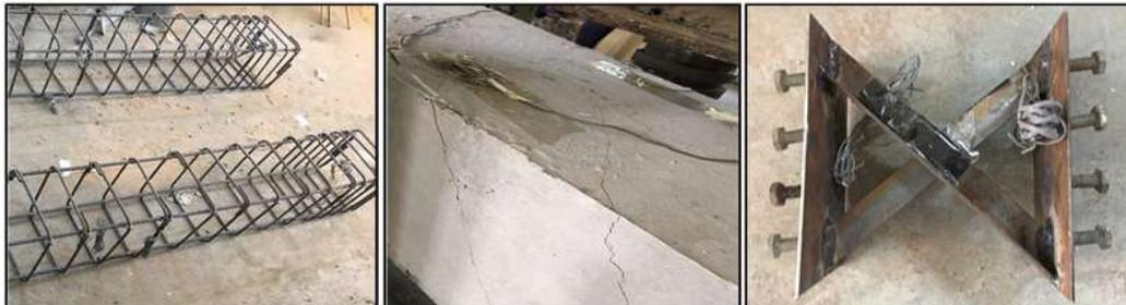
*Figure. 5 Strain Gauges in Steel bars, Steel Bracing and Concrete*
