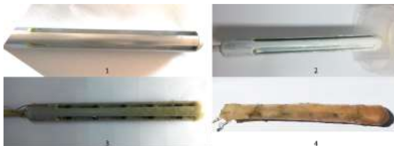
Figure 1 - Manufacture of the catheter for data capture inside the esophagus, where: (1) Aluminum with axial chamfers; (2) Mold being bathed in latex; (3) Placement of temperature sensors; (4) Final product after removal of the already hardened latex from the mold.
